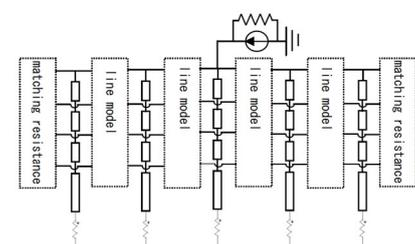
Fig.1 Transmission line model
