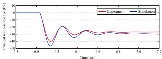
Comparison of a transient recovery voltage (TRV).
