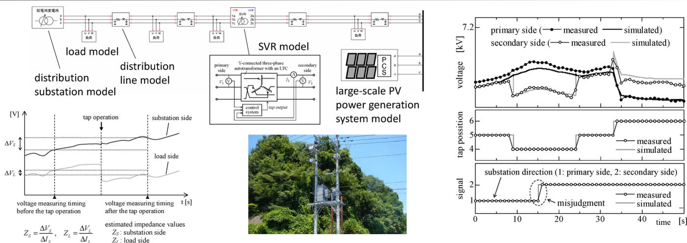
It was reported that an SVR (step voltage regulator) which is operable under reverse power flow interfered with a large PV generation system and failed to detect the substation direction. The cause has been identified by XTAP, and an improved control system of the SVR has been validated using XTAP before installation.
