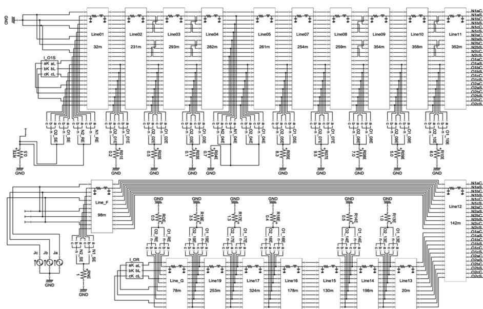
Multiple-voltage, multiple-circuit underground cable systems have been modeled in XTAP in detail so as to accurately calculate zero-sequence circulating currents. The study has solved a problem of a protective-relay malfunction.
