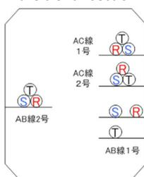
Cable arrangement in the duct section
