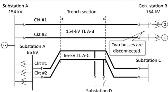
Cable arrangement in the trench section
