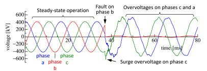
Since the EMT simulation gives detailed waveforms of all phases, momentary overvoltage and current values are obtained. It is suitable for detailed simulations of a particular part of a power system.
